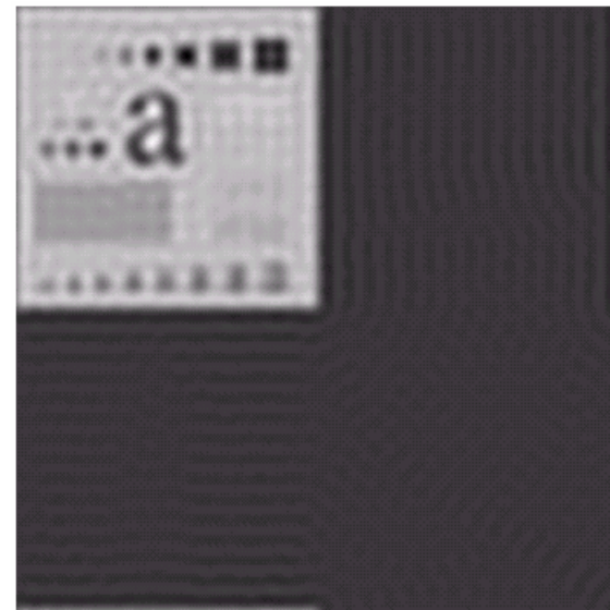
FIGURE 4.40 Result of filtering with padding. The image is usually cropped to its original size since there is little valuable information past the image boundaries.
